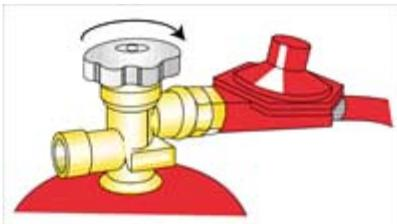
1. Turn the handwheel OFF (clockwise rotation). Wait until the burner/pilot light has gone out
