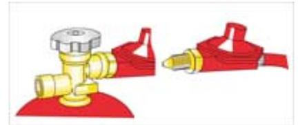
NOTE: A gas tight seal is created by face to face connection between the bullnose & cylinder valve
