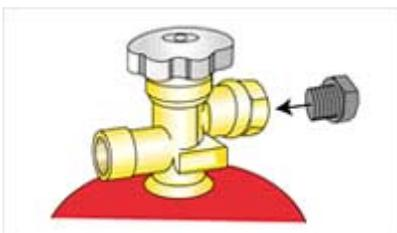
3. Close the valve handwheel OFF by turning clockwise.
